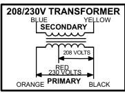
primary voltage taps as shown in figure 3, while 460 (G) and 575 (J) voltage transformers use a single primary voltage tap.
